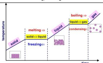
Sharp/ distinct melting and boiling points can be used to identify *pure* substances.
