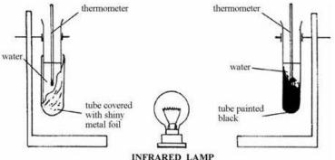
In the experiment above, the infrared lamp **radiates energy** to the test tubes. The **black painted tube absorbs** most of the energy (and its temperature increases faster) whereas the shiny foil reflected most of the energy that reached it.
